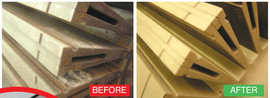
Fig 3: Turbine Generator Rotor; G&G Sponge Cleaning prior to Re-winding
