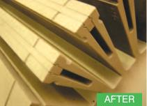
Fig 3:Turbine Generator Rotor; G&G Sponge Cleaning prior to Re-winding
